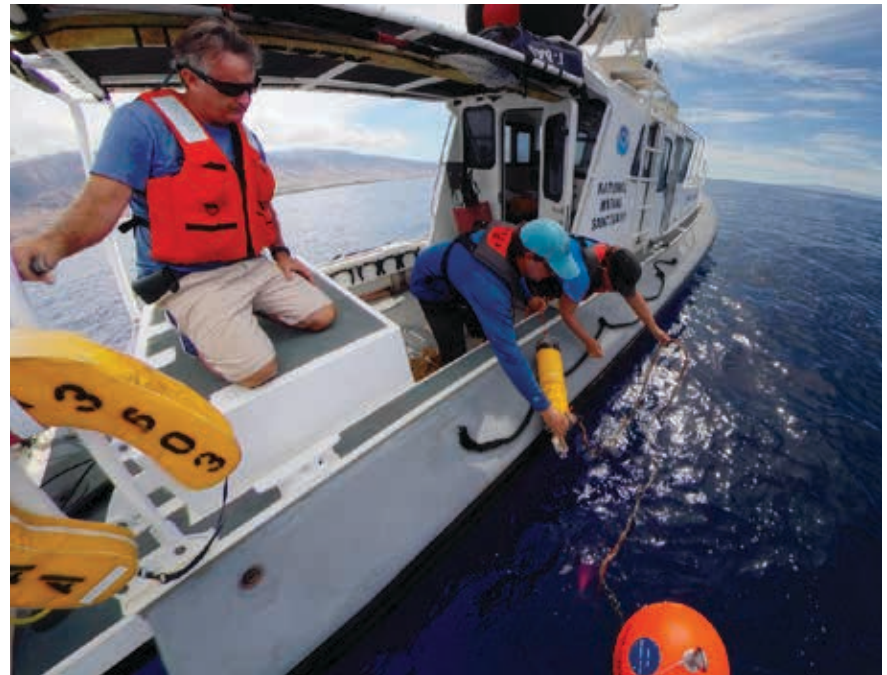
Hawaiian Islands Humpback Whale National Marine Sanctuary researchers Dr. Marc Lammers, Eden Zang, and Ed Lyman deploy an acoustic mooring from R/V Koholā. Photo by Ed Lyman/NOAA
